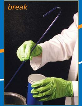
Handles are easily removed, enabling the sample to be sent away for analysis.
